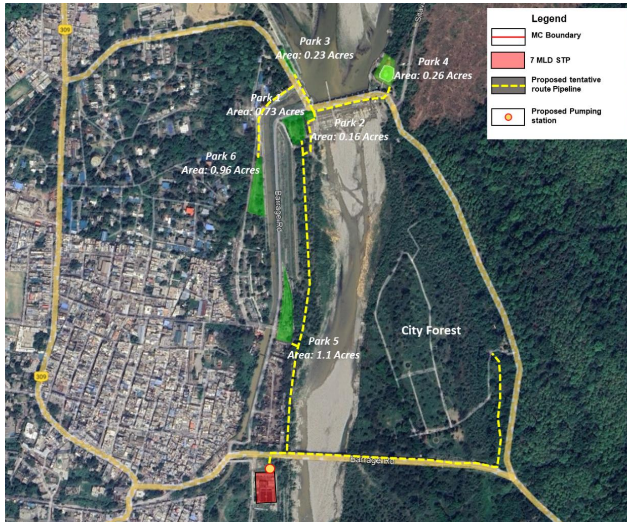
Image 7-16: Proposed reuse of treated used water from 38 MLD STP in various organized greens in close proximity
