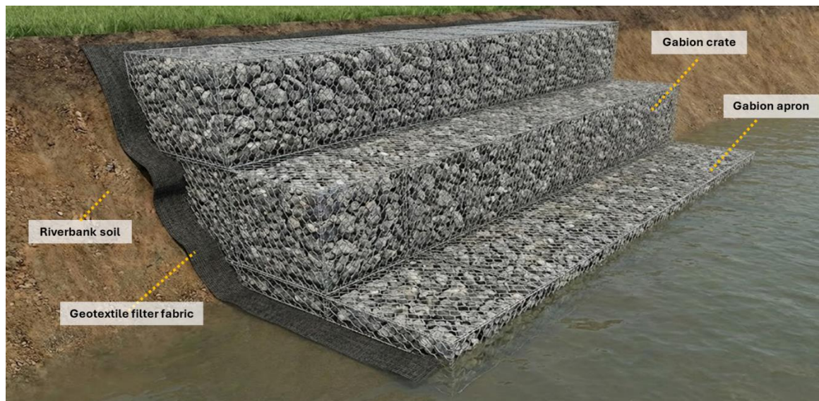
Image 7-2: Gabion bank protection measures proposed for the riparian stretch along western bank
